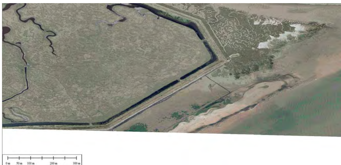
Figure 42. Aerial flown in 2001 with the consolidated bund of the recharge in the foreground. The upper right of the photo shows a natural Chenier beach which has superimposed onto the saltmarsh margins at Shinglehead Point (source: Environment Agency). A close up of the south-western extent of the natural Chenier is shown in Figure 43 below.
