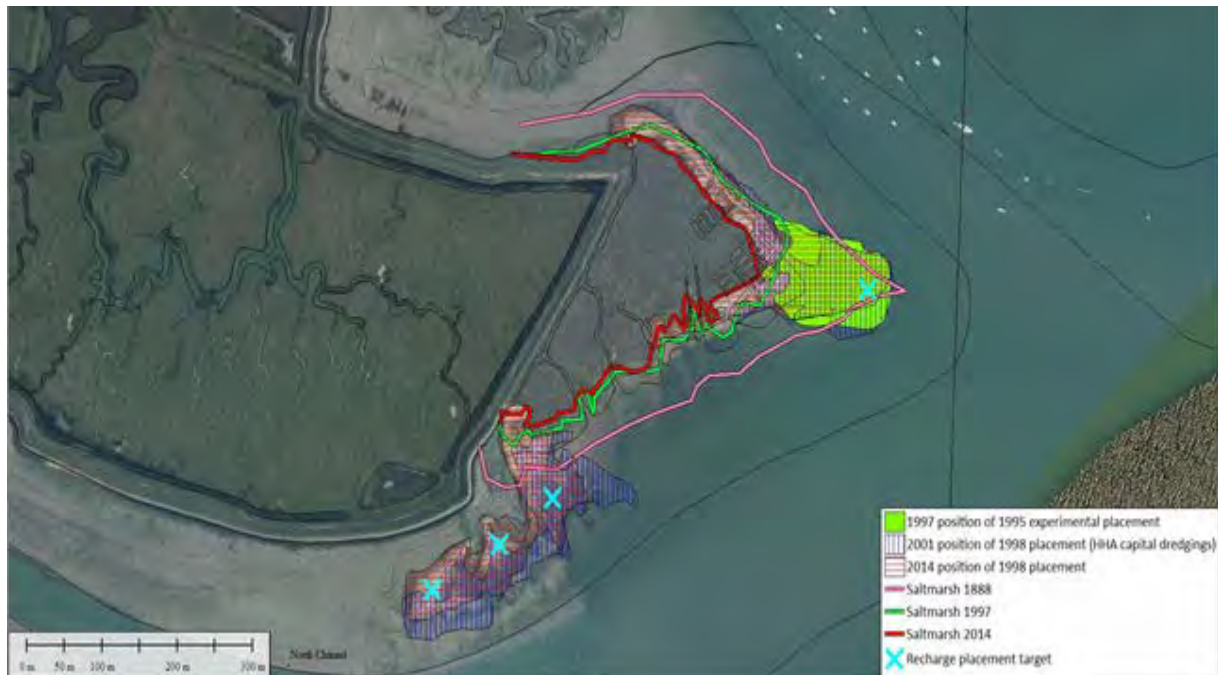
Figure 30. Shows the changing shoreline location at Old Hall Point over time and the current distribution of the recharge (2014) placed onto the eroded mudflats at the eastern quarters point and on the Tollesbury North Channel foreshore in 1998. (Jim Pullen. Source: esri satellite map & OS 1:50000 vector mapping.)
