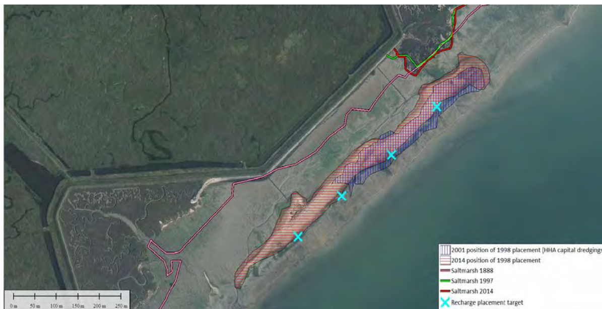
Figure 37. Indicates the shoreline along the Tollesbury Wick frontage in 1888 and compares the 2014 distribution of the recharge with the formation in 2001 following placement onto the eroded mudflats in 1999. Since 2001, though there has been some slight movement to landward, the material has remained relatively in situ. (Jim Pullen. Source: esri satellite map & OS 1:50000 vector mapping.)
