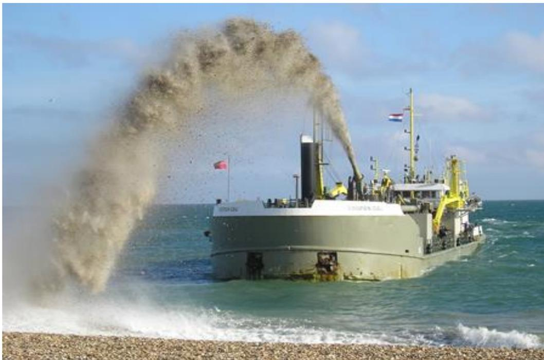
**Trailer suction dredger *Sospan Dau* that has placed previous recharge material to Mersea Harbour.**
